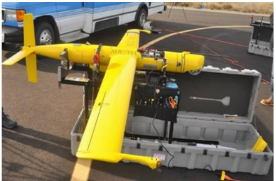
Aerovel Flexrotor storage case and integrated workbench.
